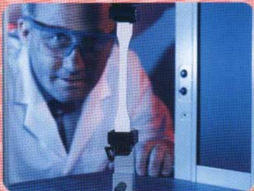
*Investigating the tensile properties of a PVC blend.*
